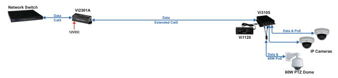
The Vi3105 can receive data over extended distance UTP up to 2,000 ft. at 100Mbps and power 60W PoE cameras using the Vi0015 combiner cable and a local power supply.
