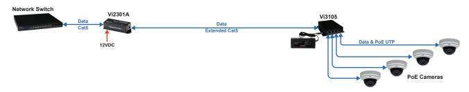
The Vi3105 can receive data over extended distance UTP up to 2,000 ft. at 100Mbps and power 4 PoE cameras using local power supplies.
