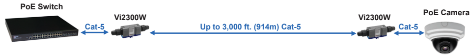
The Vi2300W can extend IP video and PoE at distances up to 3000ft.
