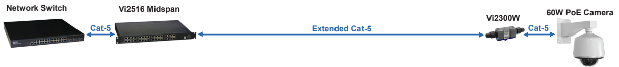
The Vi2300W can extend IP video and 60W PoE at extended distances.
